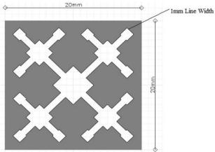
Fig. 2.Unit cell of the proposed FSS structure
