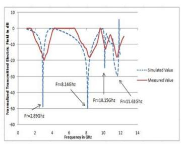
Fig. 8: Graph showing simulated and measured results of Normalized Transmitted ElectricField Vs Frequency for the designed FSS comprising of slots
