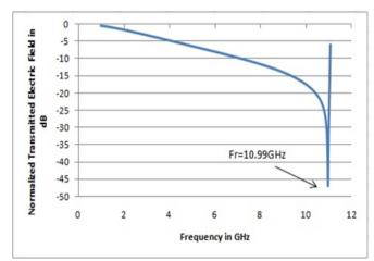
Fig 5: Study of normalized transmitted electric field vs. frequency(corresponding to Fig.1)
